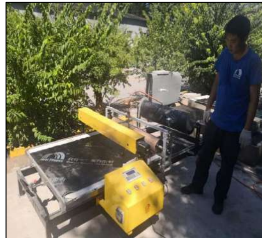
Constant hot melt testing machine for SBS modified bituminous sheet material
